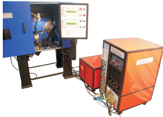
PPAW Power Source & Water Chiller / Recirculator with Engine Valve Hardfacing Automation
